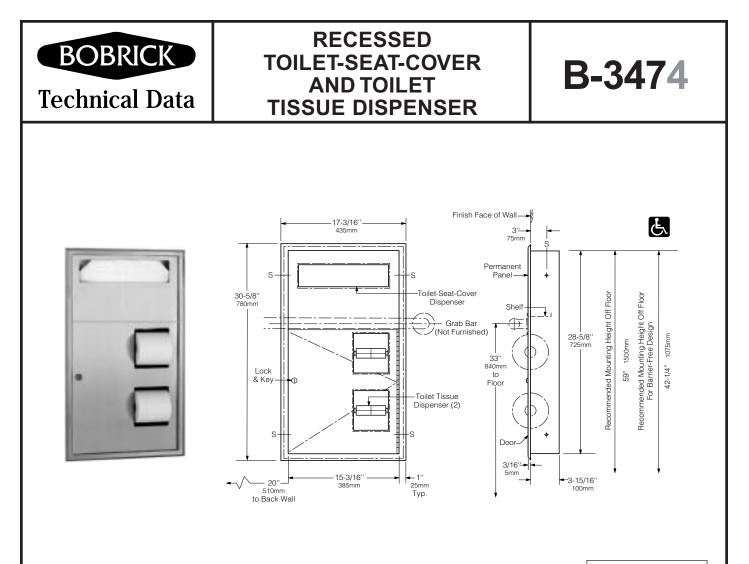
Rough Wall Opening 16" (405mm) wide 29-1/4" (745mm) high 4" (102mm) minimum recessed depth
